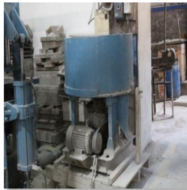
Muller mixer -2 – – to mix different raw materials for making the material
