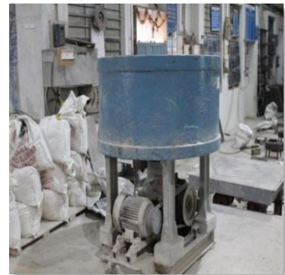
Muller mixer -2 – – to mix different raw materials for making the material
