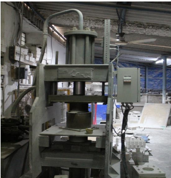
Hydraulic press (50 ton)-for small product making– small size bricks are pressed in our hydraulic press of 50 ton capacity
