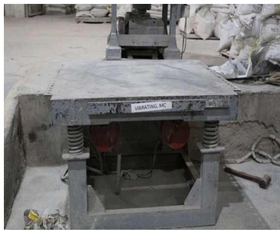
Vibrating machine-for PCPF production – this machine is used for making our pre cast & pre fired shaped bricks
