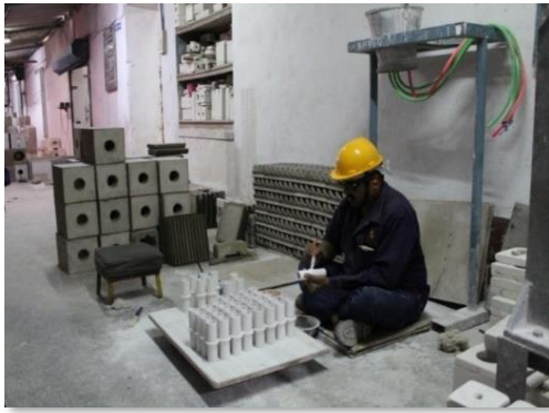
Slip cast finishing area – the ferrules are manually given finishing touches to remove any undulations or discoloration moisture
