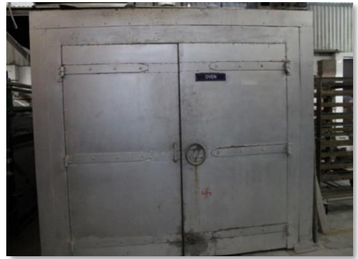
Gas oven – the bricks are dried in our gas before going for firing to remove the
