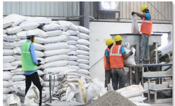
Loading the raw material into the castable machine
